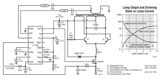
Figure 1. 14W CCFL Supply Produces a 100:1 Dimming Ratio While Maintaining Minimum and Maximum Lamp-Current Specifications
