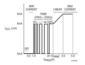
Figure 2. Lamp Current vs PROG Voltage
